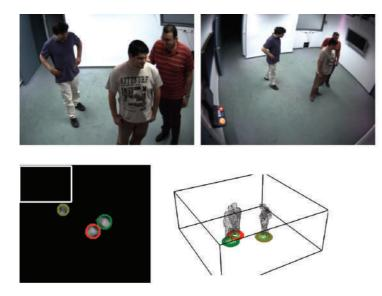
Figure 10. Person localization and tracking. (Top) Original images from two out of eight views, (below) person segmentation and 3D reconstruction. Person tracking results are rendered as circles, superimposed on the ground plane of the 3D reconstruction. Circle colors correspond to track ids. Tracking retains the correct id for all persons although it is often that visitors may come in contact or occlude each other to the cameras.
